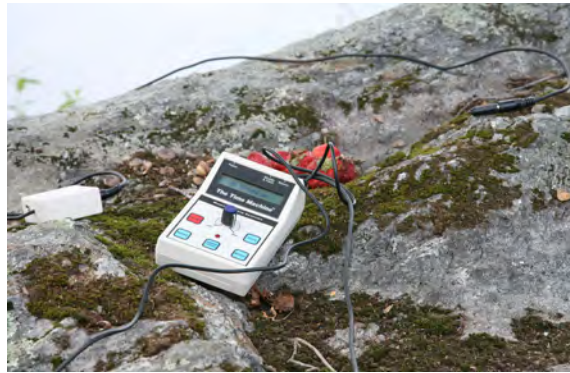
Figure 8-8: When an animal breaks the beam, The Time Machine triggers the camera.
